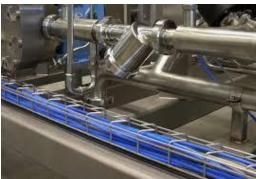
**Blue Metal Detectable Clamps:** detectable with X-ray and metal detection in case parts larger than 1MM may have come into the product. Our magnetic wire clamps have 100% chemical resistance
