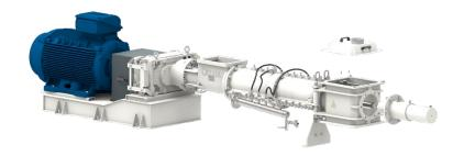
**Caption:** A real all-rounder in feed production: The expander from AMANDUS KAHL is suitable for mixing, kneading and homogenizing and ensures effective hygienization of the processed products.
